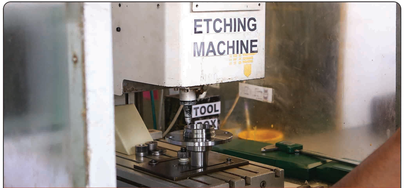
Marking Facilities Hub & Disc Assy Specification: Traceability Marking Machines
