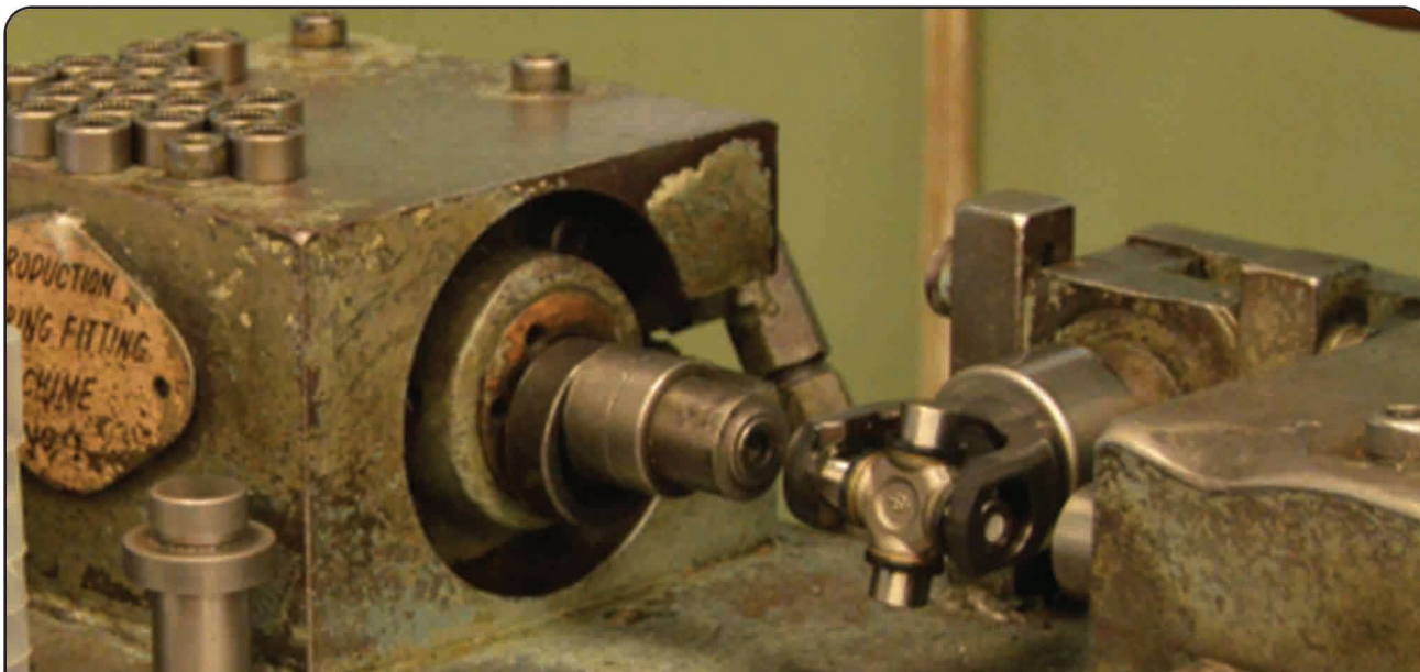
Propeller shaft Specification: Bearing Fitting press
