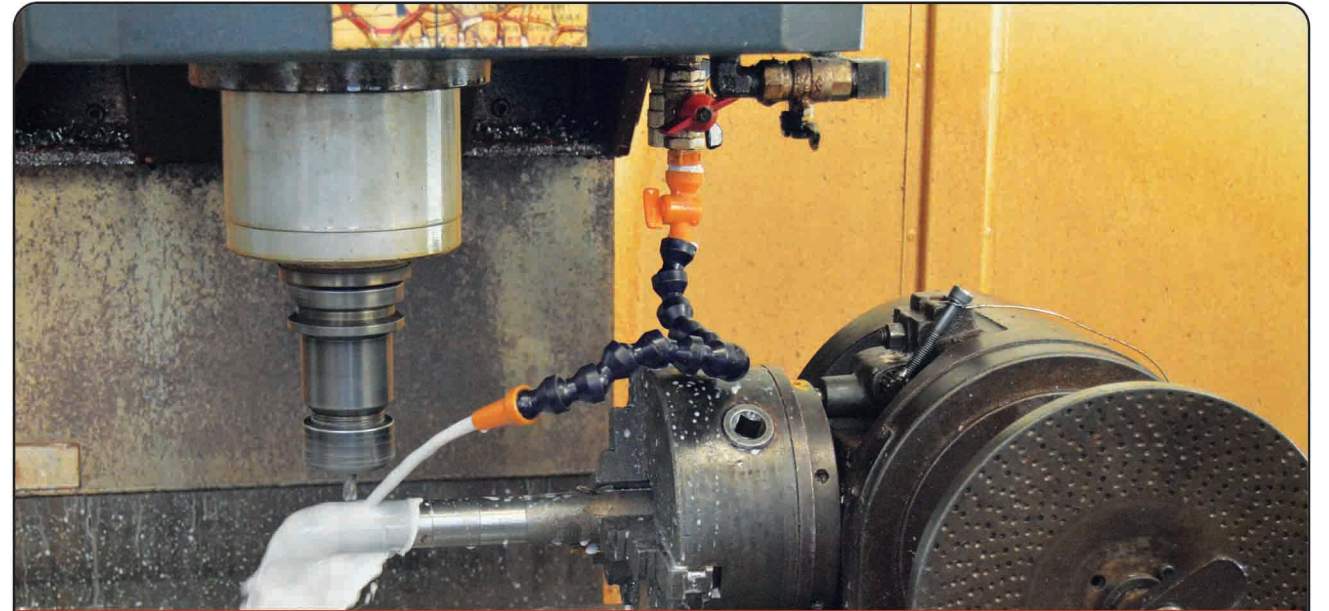
Machining Facilities Hub Front Wheel Specification: CNC Milling
